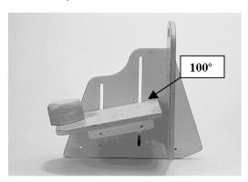
2. Adjust the angle in space. The U-shaped side frame allows the chair to be angled back in space 5°, 10°, or 15°. Remove the (4) knobs with threaded inserts and (4) nylon washers from the U-shaped side frame.
